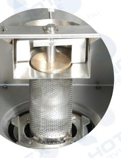
Food preparation and table waste is fed into the food waste disposer and ground into fine pieces. These are automatically washed into the dewaterer and the excess liquid pressed out. Solid waste is expelled into a bin from the discharge chute. Liquids are flushed down the drain or recirculated in the system.
