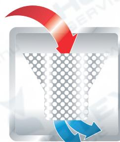
The fine filter system GENIUS-X<sup>2</sup>, with integrated pre-washing process, filters the wash water continuously and then pumps out the soil particles.
